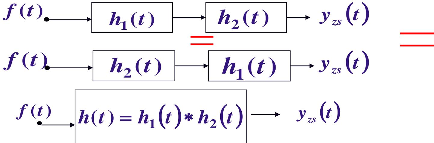
$$\because [f(t) * h_1(t)] * h_2(t) = f(t) * [h_1(t) * h_2(t)]$$
