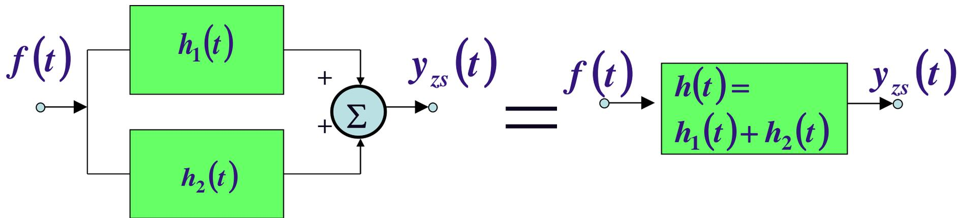
$$\begin{aligned} y_{zs}(t) &= f(t) * h_1(t) + f(t) * h_2(t) \\ &= f(t) * [h_1(t) + h_2(t)] \end{aligned}$$
